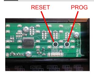
With the device powered, press and release the RESET button.
